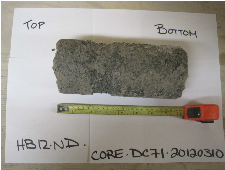
Photo 19: HB12-ND-CORE-DC71-20120310 drilled on dayshift around the time of freeze back in area.
