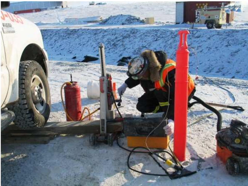
Photo 4: Coring previously placed FCM
