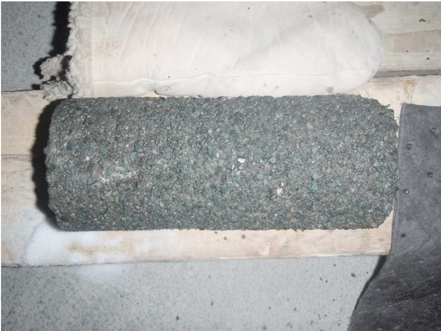
Photo 20: HB12-ND-CORE-DC72-20120310 drilled on Nightshift around 0+90 CL, immediately after freeze back in this area.
